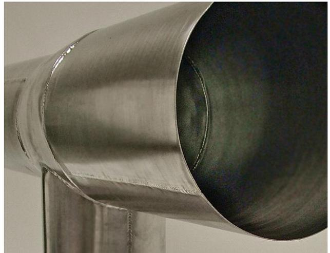
**Fabricated chamber made of iridium sheet**
