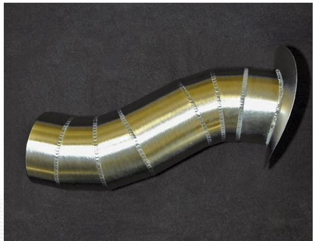
**Fabricated tube made of platinum/rhodium sheet**
